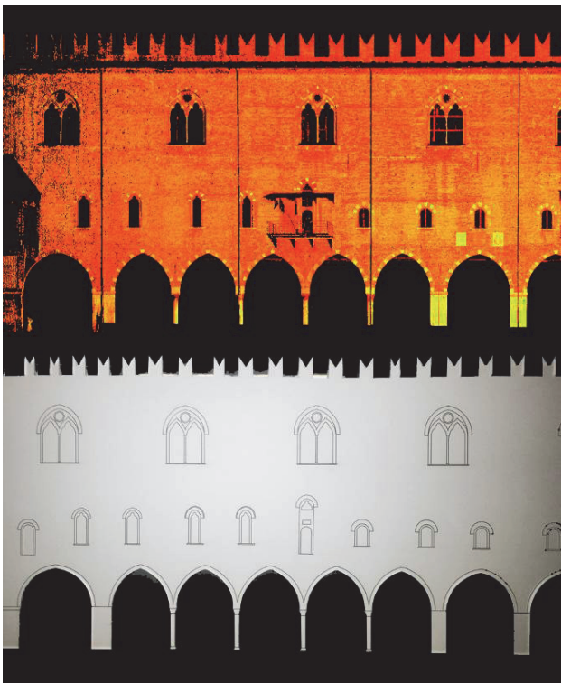
Fig. 5. The process for the construction of the physical model: orthophoto from laserscanner, facade drawing and simplification.
