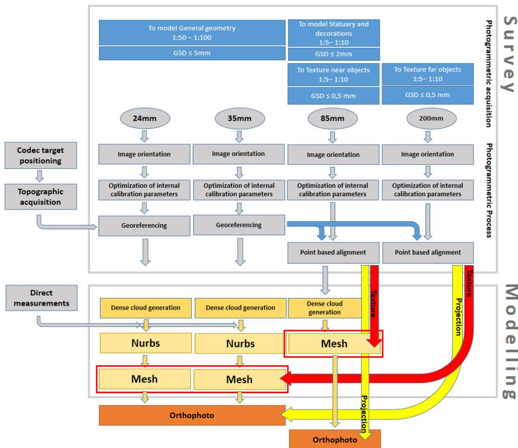
Figure 8: Diagram of the survey and modelling phase.
