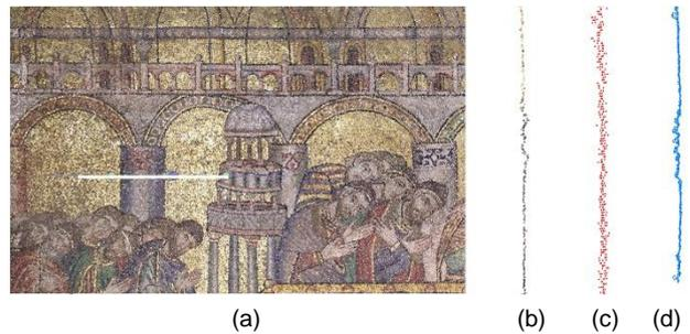
Figure 6: Analysis of the point cloud resulting from the laser scanning survey: comparison between the scanner and the photogrammetric survey: a) detail of the mosaic surface; b) profile extracted from the photogrammetric cloud; c) profile extracted from the Leica C10; and d) profile extracted from the Leica HDS7000.
