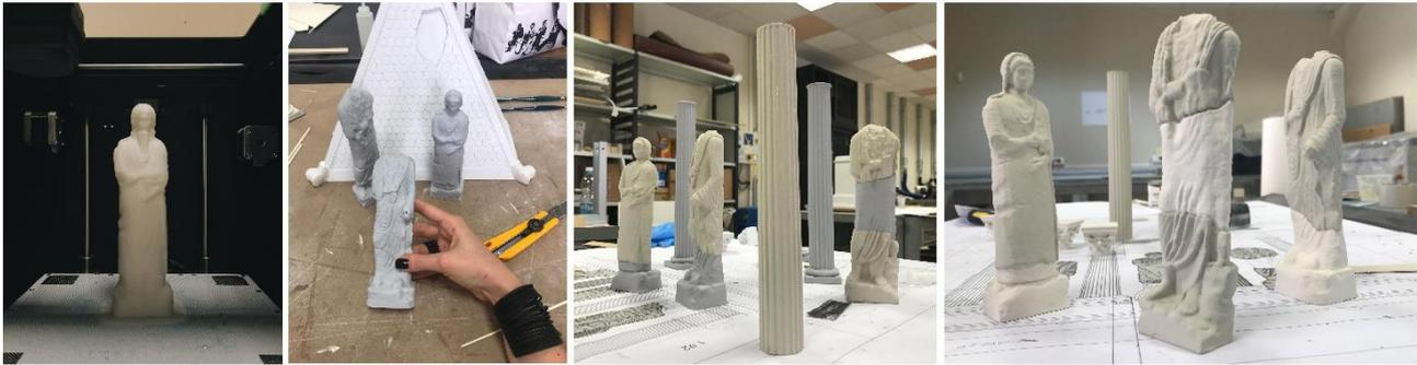
Figure 3: sequence of statues (3D printing, post-production, final finish)
